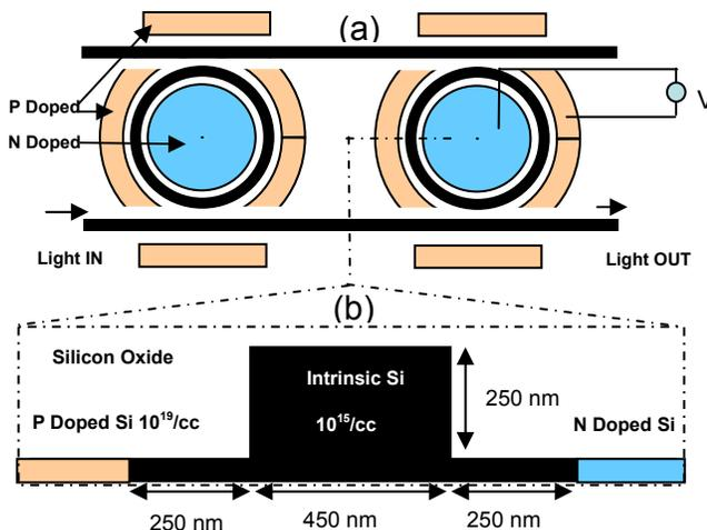
Fig. 1: a) top view schematic double ring resonators embedded in PIN diodes
