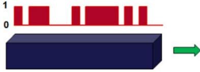
Fig. 7. Bandwidth density: the bandwidth density of the waveguide is given by the aggregate data rate in the waveguide divided by the separation of two consecutive waveguides in an array of waveguides.
